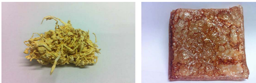
Figure 1. Photographs of the dried SPEEK products obtained after precipitation in cold water under two different mixing conditions: gentle stirring with a mechanical stirrer (left) and vigorous stirring with a glass rod (right). [Color figure can be viewed in the online issue, which is available at wileyonlinelibrary.com.]
