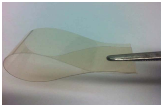
Figure 3. Photograph of the as-prepared 3c-SPEEK. [Color figure can be viewed in the online issue, which is available at wileyonlinelibrary.com .]
